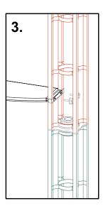
Hand tighten thumb screws into the bracket holes.
