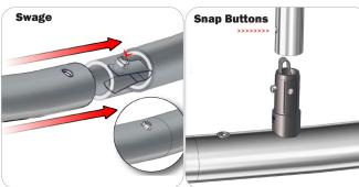
Locate the snap button on the connector or swage tube. Locate the hole on the corresponding tube. Press the snap button with your thumb and slide the tube and connector together so that the snap button snaps fully into the lock hole. To disassemble, press the snap button and pull apart.
