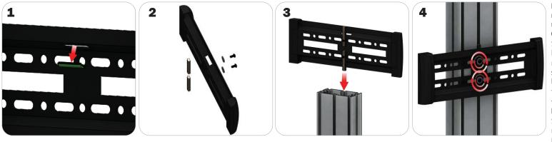
TRI-30MM Channel Tube Connection
