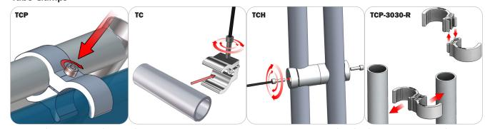
Be sure to fully assemble all frames before using clamps. With the clamp unlocked, place one tube of the first frame into the mouth of the clamp. Place the second tube (if applicable) into the second mouth of the clamp. With both frame's tubes in the clamp, be sure to lock securely, but do not overtighten.
