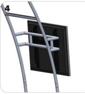
Locate all components needed to assemble the monitor mount with the TRI-30MM Channel Tube Connection method. You will need (1) monitor bracket, (2) Square Bolts, and (2) Wingnuts.
