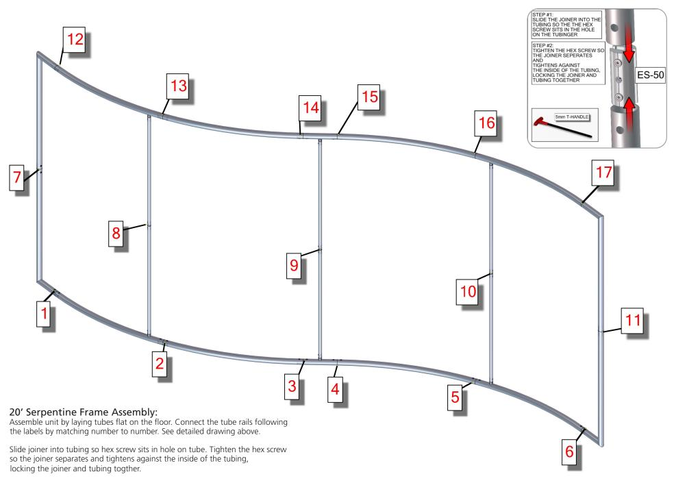
At connection 8, 9 and 10, connect tubes by pressing snap on button, lining up holes and securing button in hole.
