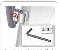
Secure second tube clamp TC-30 around backwall and tighten with 3/16" hex key tool.
