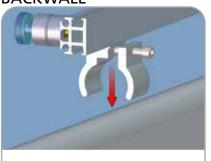
Once graphic is attached to stand-offs and extrusion, position tube clamps (TC-30) onto backwall.
