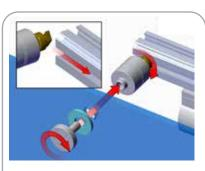
Attach graphic to stand-offs and extrusion with washer & other end of stand-off. Turn clockwise to secure.
