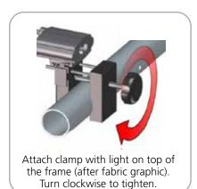
STEP 10: ATTACH LADDER TO BACKWALL WITH CLAMPS
