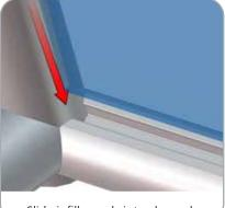
Slide infill panels into channels.
