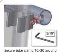
Secure tube clamp TC-30 around backwall at desired height and tighten with 3/16" hex key tool.
