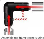
Assemble top frame corners using TC-30-90. Label codes will be on backside of tube. It is best to assemble frame laying flat.
