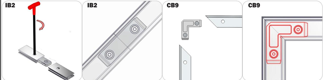
Press the hex bolt head in with your thumb and slide the extrusion and connector together so that the hex bolt head sits into the lock hole. Repeat with the second extrusion to the free end of the connector. Lock the extrusions together by turning carefully with the allen key tool. Be sure to lock securely, but do not overtighten.
