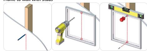
First, find the wall studs and mark it with a pencil. You can use a stud finder to help locate the studs. Second, drill holes on the frame for screw clearance. Do not make the holes larger than the screw heads. Make sure to drill on center for top and bottom horizontal frame runs. Third, level and hold the frame in place lining up the frame holes with the pencil line. Finally, use a hand screw driver to secure the frame onto the wall with the provided screws.
