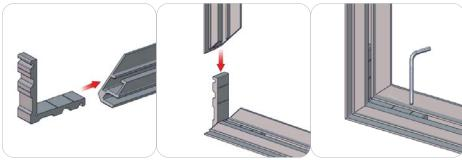
First, insert the corner connector into the extrusion. Then, slide the next extrusion onto the same corner connector. Finally, hold the corner components together and use the provided Allen Key to lock the corner connector in place.
