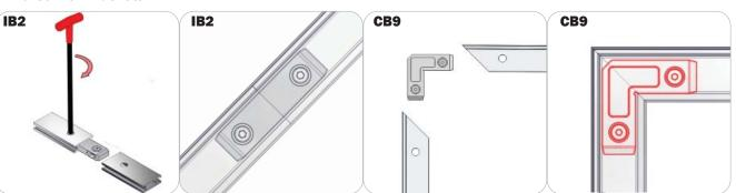
Press the hex bolt head in with your thumb and slide the extrusion and connector together so that the hex bolt head sits into the lock hole. Repeat with the second extrusion to the free end of the connector. Lock the extrusions together by turning carefully with the allen key tool. Be sure to lock securely, but do not over tighten.
