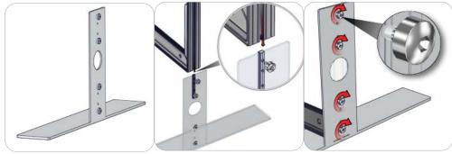
An SW-FOOT assembly consists of two thumb screws, an LN100, and SW-FOOT baseplate. Start by loosening the thumb screws (it is best not to completely remove the screws). Slide the extrusion onto the LN100 by utilizing its back cam channel. When the extrusion rests on baseplate or ground (depending on application), tighten the thumb screws to lock in place. Do not over tighten.
