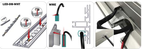
Be sure to fully assemble all frames before using the internal lighting components. With the thumbscrews loosened, place the light strips on the frame, then hand tighten them in series, male to female connections with extension cords. Do not over tighten the thumbscrews. Snap on the wire management extrusions with the power cord extensions in place. Reference the Internal Lighting Diagram for more details.
