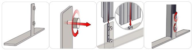
An SW-FOOT assembly consists of two thumb screws, an LN100, and SW-FOOT baseplate. Start by loosening the thumb screws (it is best not to completely remove the screws). Slide the extrusion onto the LN100 by utilizing its back cam channel. When the extrusion rests on baseplate or ground (depending on application), tighten the thumb screws to lock in place. Do not overtighten.
