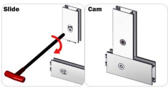
A cam lock equipped extrusion can lock to any cam lock channel. With the cam lock unlocked, set the teeth of the cam lock into the desired position on the cam lock channel. Using your allen key tool, carefully turn the lock clockwise to lock in place. Be sure to lock securely, but do not overtighten.
