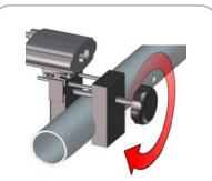
Attach clamp with light on top of the frame (after fabric graphic). Turn clockwise to tighten.
