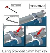
Using provided 5mm hex key, rotate bolt clockwise to secure accent to top of fabric backwall.
