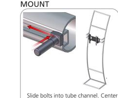
Slide bolts into tube channel. Center monitor mount on hardware.
