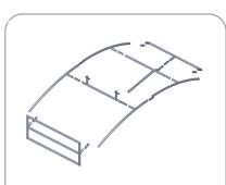
Connect bottom and top tubes following the labels, then connect side tubes. Note tubes with velcro on face,
