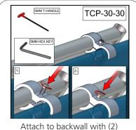
Attach to backwall with (2) TCP3030 back to back tube clamps.
